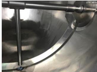
INOX Aseptic horizontal surface sweeping agitator for viscous product with particulates
